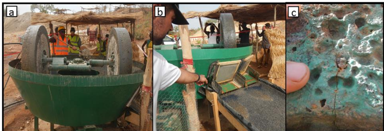
Figure 5: a) Mill/Slucifier system showing the mill to sluice to tailings pond flow. b) Dust cloud produced from the batch and disk mills currently used by workers on site.
