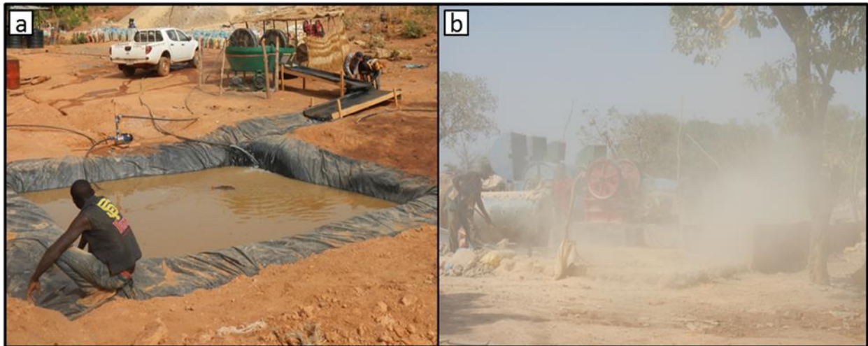
Figure 5: a) Mill/Slucifier system showing the mill to sluice to tailings pond flow. b) Dust cloud produced from the batch and disk mills currently used by workers on site.
