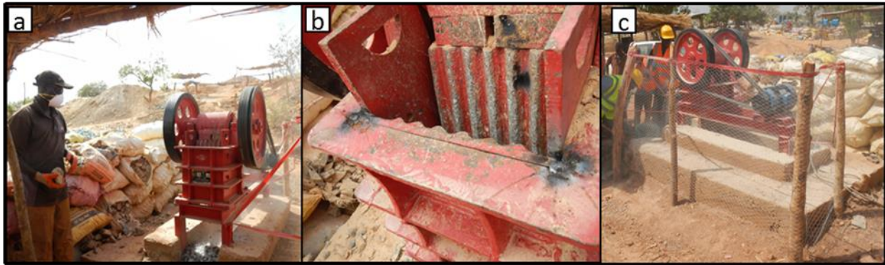
Figure 4: a) Worker hand feeding ore into the crusher. b) Close up view of jaws and weld. c) Side view of jaw crusher with safety fence protecting motor and belts.
