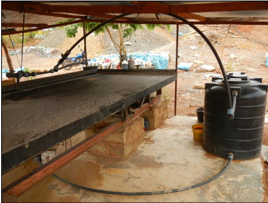
Figure 9: Shake table and associated water system showing table, polytanks, water inputs to the slurry and water troughs, and water return pipe.
